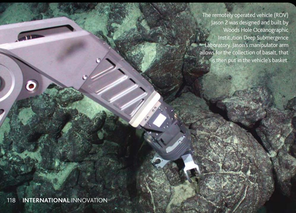
The remotely operated vehicle (ROV) Jason 2 was designed and built by Woods Hole Oceanographic Institution Deep Submergence Laboratory. Jason's manipulator arm allows for the collection of basalt, that is then put in the vehicle's basket.
